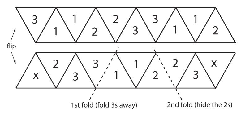
This diagram shows how to label the triangles on each side of the strip. Once you have made this strip and creased each line both ways, make the 1st fold then the 2nd fold as shown, so that each face has the same number on all triangles. Tuck the last part behind, and fold the flaps marked x together and glue the faces with x on to each other.
